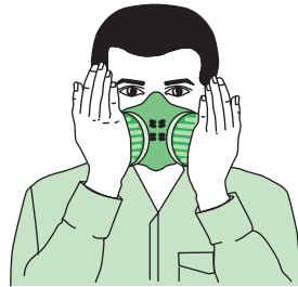
Negative pressure seal check
