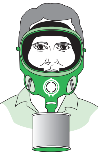
Gas mask with canister (TC-14G).
