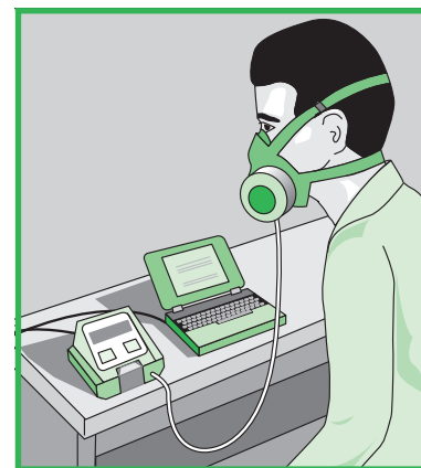
In a quantitative fit test, a particle-counting instrument is used to measure respirator fit.
